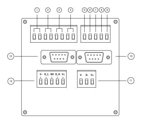
Figure 2 - Terminal Blocks and Connectors
